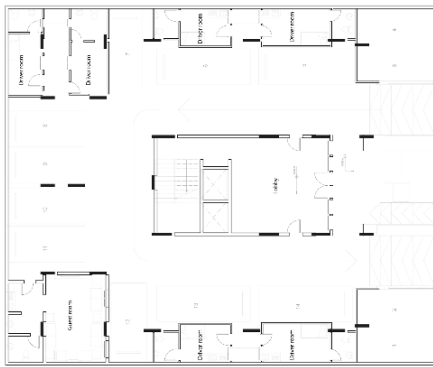
Figure 1.3.a First floor plan (ground floor) (14 Parking spots, 6 Driver rooms, and 1 guest room).
